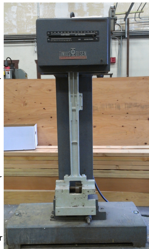
Picture 2. Charpy V-notch machine.
