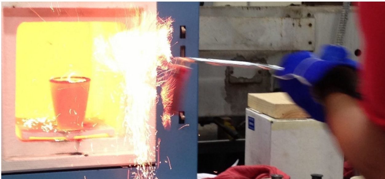
Picture 1. Removal of heated sample from oven at 980°C .
